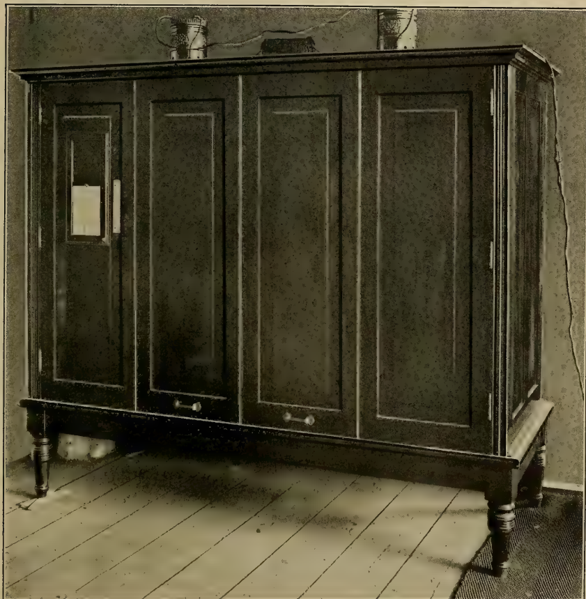
PLATE 219.—This Plate shows the Arc-Light Bath Cabinet as it appears when closed with patient inside. The thermometer near the observation window records the temperature during treatment, and this usually reaches 95 to 100 degrees F. Each section of the front is removable, and on casters the apparatus can easily be rolled to any part of a room.
